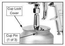
Figure 4. Installing cup.
